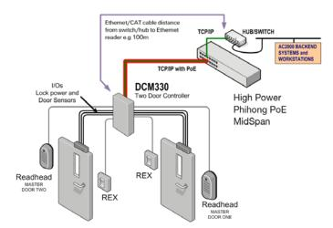
The PoE+ injector or mid span device supplies all the power for the devices and locks required by two doors.
