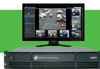
The AC2000 video interface for American Dynamics Hybrid Video Recorders (HDVR) provides the ability to associate access control alarms with digital video clips and to view live camera footage. This enables AC2000 to act as the central Security Management System (SMS).
