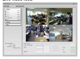
The operator can split the video screen into 1x1, 2x2 (4), 3x3 (9), or 4x4 (16) options allowing the operator to view live video feeds from up to sixteen cameras simultaneously, each in its separate pane. Each pane can be simply configured using a drag and drop facility to place the appropriate camera into the required pane, this can then be saved allowing instant viewing of the configured matrix each time the application is opened.
