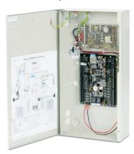
The CEM DCM 350 (Door Control Module) is a low cost, two-door controller that is designed to interface to CEM sPass DESFire smart card readers. By utilising encrypted RS485 serial communications between the eDCM 350 controller and the sPass reader, the threat of Wiegand controller signal cloning is effectively eliminated. The DCM 350 is available in two options-the sDCM 350 supports serial devices while the eDCM 350 supports IP devices.
