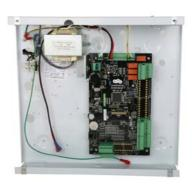
The Ethernet Input Output Controller (EIOC) is an addition to the Ethernet suite of devices for use on the AC2000 system. Connecting to the nearest network point the EIOC provides a flexible means to monitor and control an array of equipment. The EIOC features 16 analogue inputs and 8 digital outputs. The 16 analogue inputs can be cross-mapped to one or many of the outputs upon activation/deactivation.
