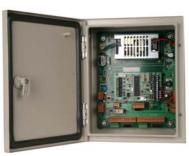
The DIU 200 and DIU 210 door interface units are designed to provide power to a door lock, as well as local power to a CEM reader. It has onboard inputs which can be used to monitor conditions such as a fire alarm or activated break-glass condition.
