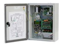
Used in conjunction with the S9032, the AC2000 Lift Control Interface (LCI) allows seamless control and monitoring of access between elevator floors. An LCI unit directly connects to a lift floor selection panel. The LCI unit outputs activate buttons on the lift floor selection panel according to the access permissions of the card holder. LCI inputs then record which button was pressed.
