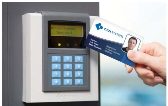
control panel in the system design. With an internal database, the S610e gives full off-line card validation and decision making at the point of entry, even when host communication is not available.
