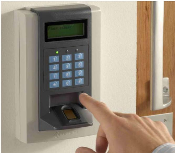
The S610f has a large internal database which holds card and encrypted biometric templates at the door. This ensures zero system downtime at air-bridges. The S610f also features an LCD screen to show personnel meaningful user messages and has many airport specific door modes such as 'Passenger Mode' and 'Lobby Mode' for extended door open times at air-bridges. With S610f readers in place, only authorised and trained personnel can use the air-bridges.
